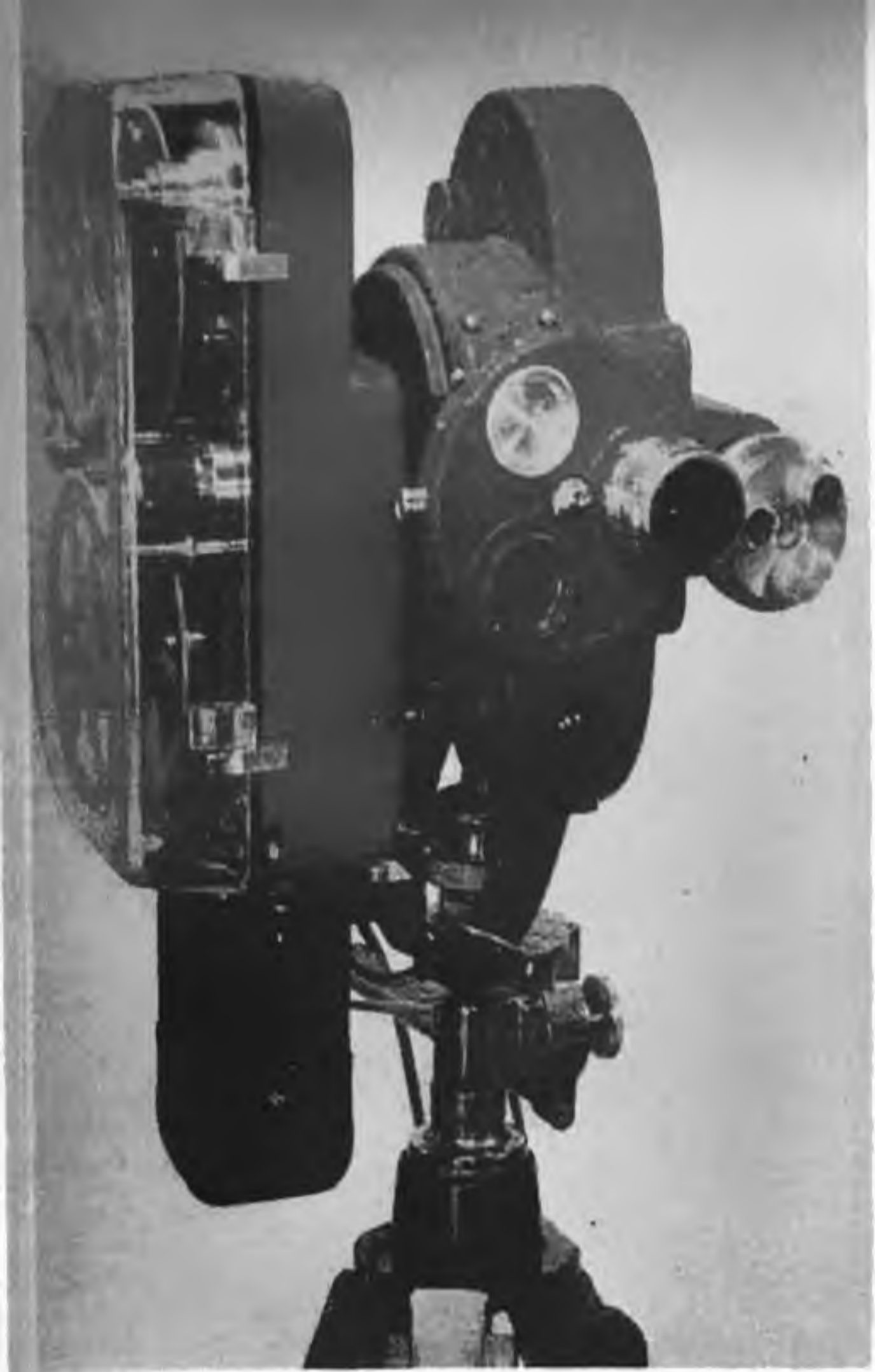
The Synchronflex on a Bell & Howell 70 camera—a very simple fitting job though slightly more noisy in operation than with the Bolex.
