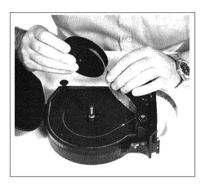
It is important that the film which is slid under the hooks (d) of the sprung pressure plate forms equal sized film loops before and after the pressure plate. (When the magazine is placed on the camera the hooks are no longer in contact with the film).
