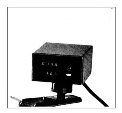
separated from its battery. The EFC-16 SR can be connected directly via a cable with the camera's electronic shoe. (Socket 45); when the VSU is used with the EFC-16 SR, the accessory distributor ZV is necessary. The counter is attached to the additional thread (40) on the camera carrying handle; the ball and socket joint connection enables the EFC-16 SR to be positioned in any direction for easy reading.
