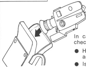
Make sure that the camera is put into the camera case only **with the lens first**. This is the best way to protect the camera from damage.
