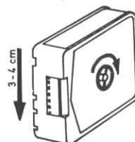
Remove the cartridge and push the film forward manually by few inches — wind by hand in the direction of the arrow (see Illustration). In addition, loosen the film windings by knocking gently against the cartridge.
