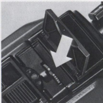
The f/stop setting can be seen low in the viewfinder. A red warning sign appears right below the f/1,2 setting when it is too dark for filming. In this case either use a movielight or a high-speed film.
