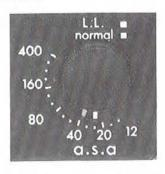
To shoot in dim light, e.g. indoors, or to have more depth of field outdoors, pull variable shutter control 8, set it to its "LL" (low light) position and push it back. Then bring
