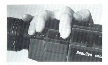
It is sometimes wiser, when hand-holding the camera, not to zoom all the way to telephoto, as it might result in unsteady pictures. So the Schneider zoom is fitted with a switch which automatically stops zooming at 40 mm ("6-40" position).
