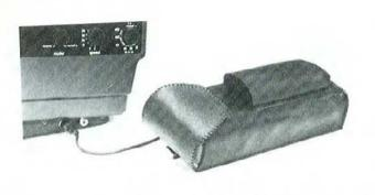
Accepts 6 R 14-type, NiCad, 1.2V batteries and connects with the "9V" socket of the camera (see page 29). Those R 14-type batteries are supplied uncharged. Charging them is possible from the specially designed charger.
