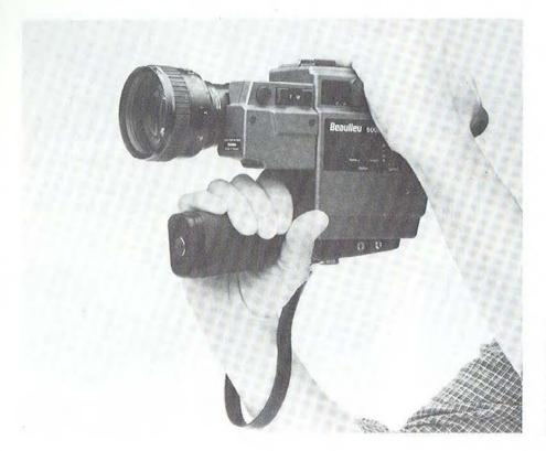
The picture above shows how you should hold the camera when filming. You power and release the camera with your right hand. The strap around your wrist will avoid accidentally dropping the camera.
