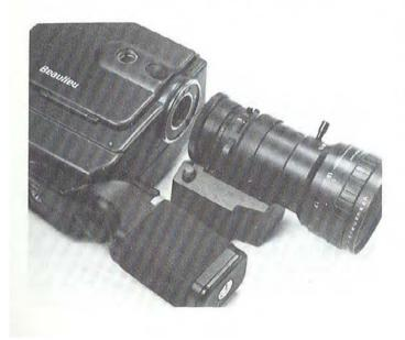
lens. Hold the lens firmly and position it onto the camera, with diaphragm servocontrol **3** on the left side. Secure the lens by tightening ring **25**.
